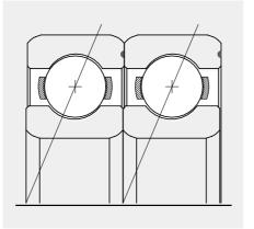
Matched bearings are usually matched with a defined preload. A specified axial clearance (GUA) or universal matching (GU) is possible for G1- and G2- bearing sets on request.
